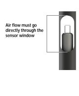
The Series 490 is calibrated for use in air. Gas correction factors for gases other than air are available from third-party sources. Note that gas correction factors can vary from meter to meter.
