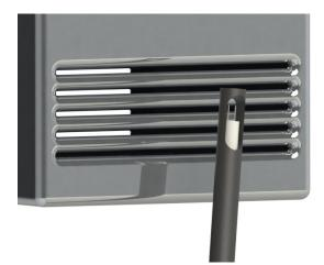
Air flow must go directly through the sensor window
