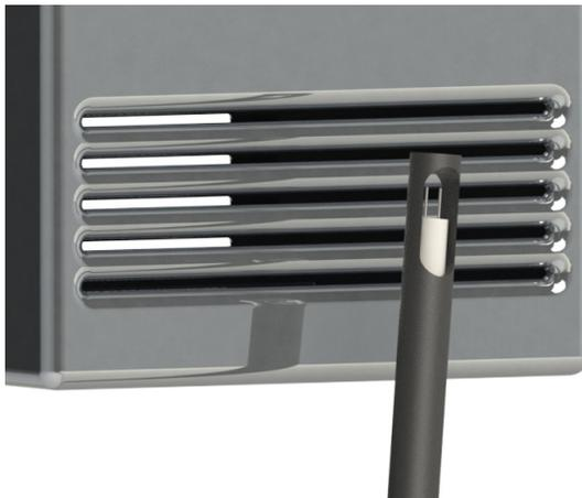
Air flow must go directly through the sensor window
