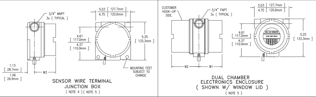
TABLE 1 SERIES 504FTB IN-LINE MASS FLOW TRANSMITTERS DIMENSIONS
