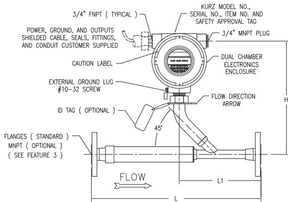
DIRECTLY ATTACHED ELECTRONICS ENCLOSURE ( TA )
