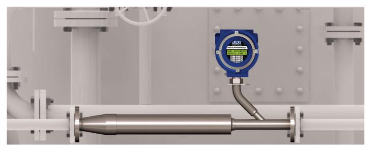
The Kurz 534FTB is designed with built-in inlet and outlet piping reducers/expanders to produce exceptional immunity to upstream and downstream flow disturbances caused by elbows, valves, and line size changes.
