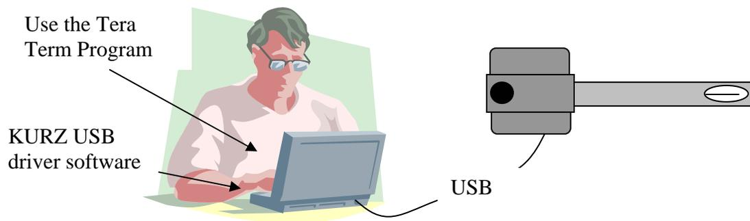
On the PC start a terminal emulator program like Tera Term, then using the lower case c, d, p, enter and other keys to navigate the menus and make changes. If it is not already echoing the LCD display, you start/stop the communications with the + key and will see a dialog like shown below. The unit shown below had its Echo turned on where a list of terminal commands was shown then it started scrolling its meter data with their tags.
