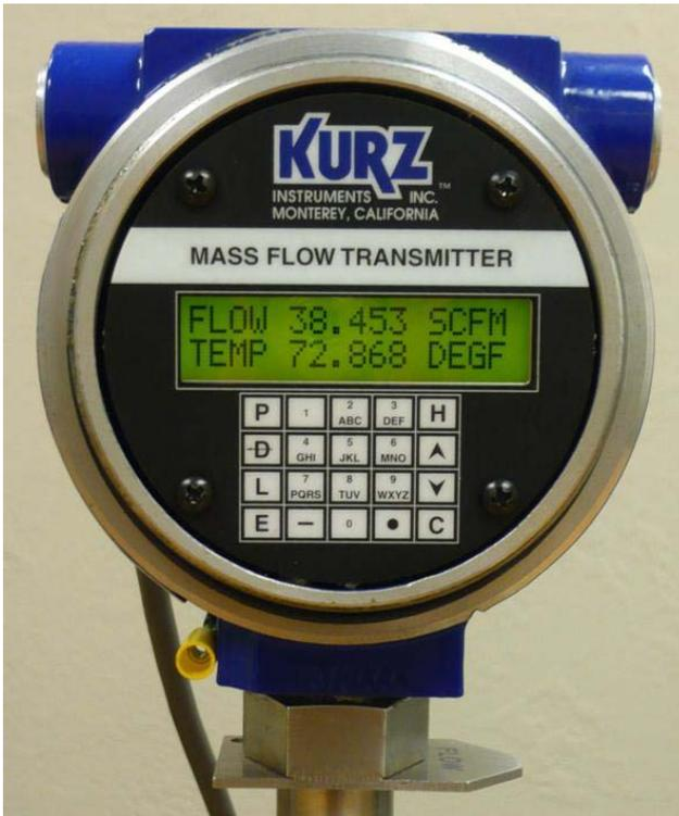
The primary keys on the keypad used to navigate the menu system are the P, D, L, E, and H keys. The remaining keys are primarily used for data entry. A PC/laptop running a terminal emulator program such as TeraTerm can be used instead of the onboard keypad and LCD display. The corresponding navigation keys on the remote keyboard are the lowercase (non- shifted) p, d, l, h keys and the ENTER key functioning as the E key on the meter keypad. The Table below defines the functions of the keys
