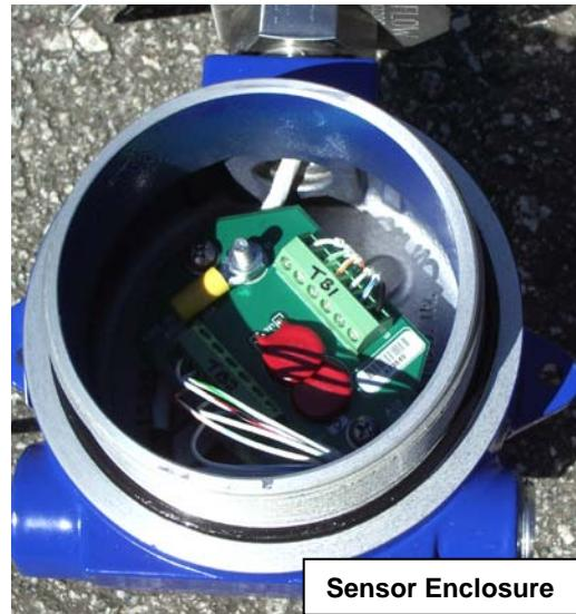
Figure AH-3. Sensor electronics enclosure and sensor J-box with covers removed
