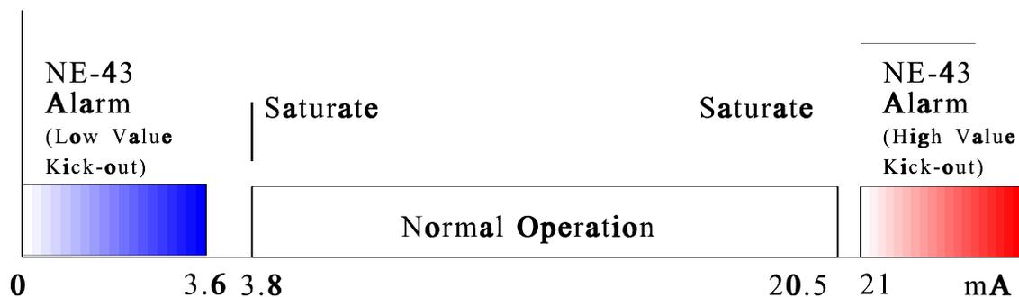
Figure F-1 4-20 mA operation with the NE-43 alarm.
