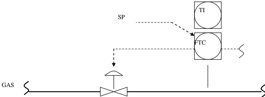
The example above has the MFT B-Series flow meter actuating a valve based on an external set point of the flow rate. The second 4-20 mA output channel is sending the flow rate signal elsewhere, although it could be temperature instead of flow rate. PID control of the process is manually configured. The control output may be controlled manually from the LCD display to verify the range operation of the control loop or to manually set the output (control valve) at a fixed position.
