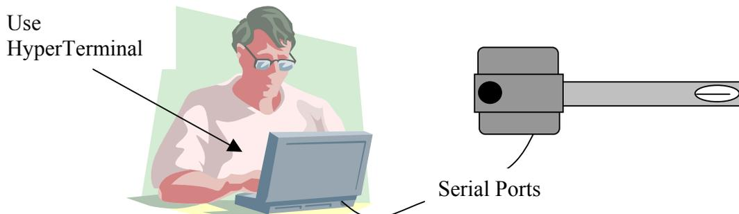
On the PC or PDA you start a terminal emulator program like HyperTerminal, then you can use the lower case c, d, p, enter and other keys to navigate the menus and make changes. You start/stop the communications with the + key and will see a dialog like shown below on a MFT unit. The unit shown below had its Echo turned on where a list of terminal commands was shown then it started scrolling its meter data with their tags.
