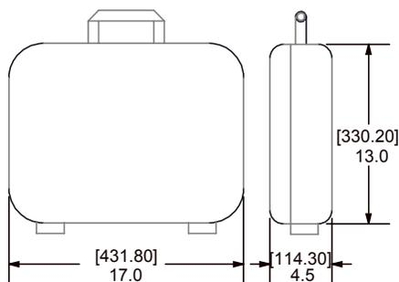
CARRYING CASE FOR MODELS WITH PROBE SUPPORT LENGTHS 48" TO 60"
