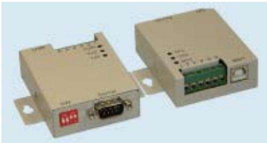
Desk computers and laptops can interface to the RS-485 devices using a USB dongle converter. We recommend the industrial version from [EasySync](#), available from Kurz (PN 700491) or the manufacture. This device is optically isolated, screw terminal interface with metal enclosure and status LEDs, with a biased bus allowing the auto-polarity detection to work.
