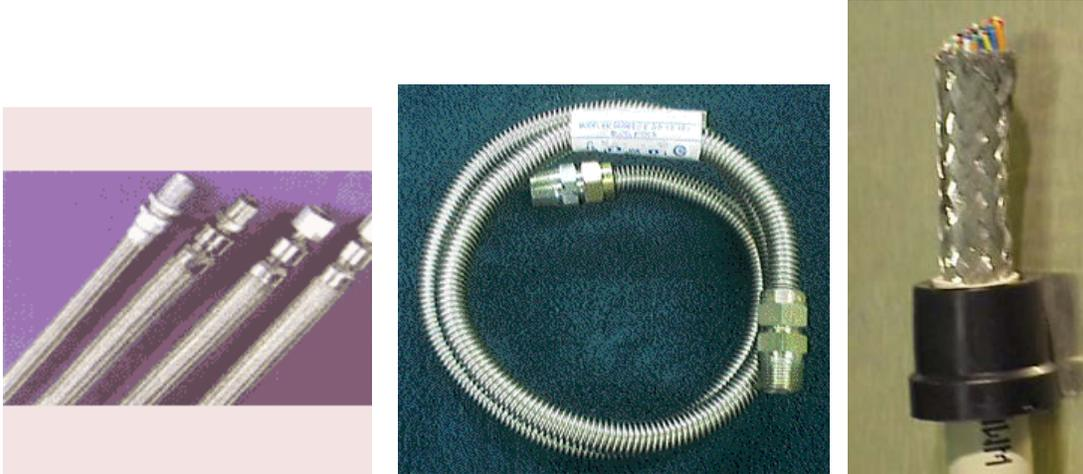
Figure A-6. Metal Braid Hydraulic Lines, corrugated gas appliance line and braided shielded cable all work well for EMC shielding of 5-wire sensor connections.
