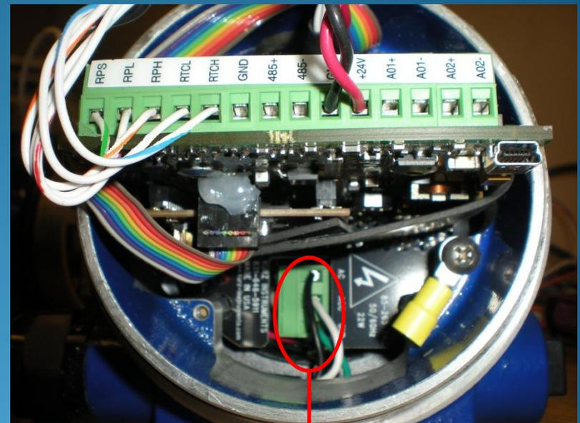
AC power field wiring installed
