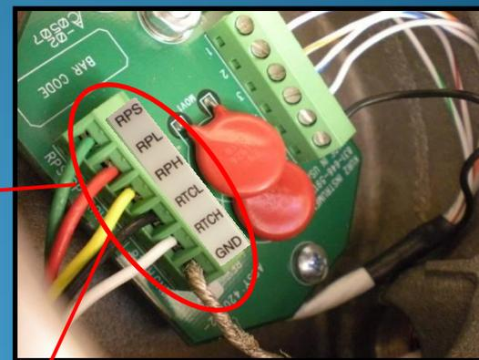
The sensor wires should terminate at the electronics enclosure and the sensor enclosure at the terminals marked RPS / RPL / RPH / RTCL / RTCH as shown and the braided shield should terminate at the GND terminals
