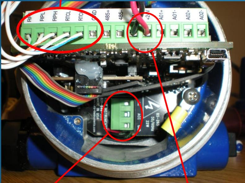
Terminal strip for customer's AC power input
