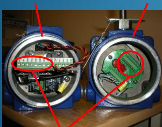
Terminal connections for sensor wiring
