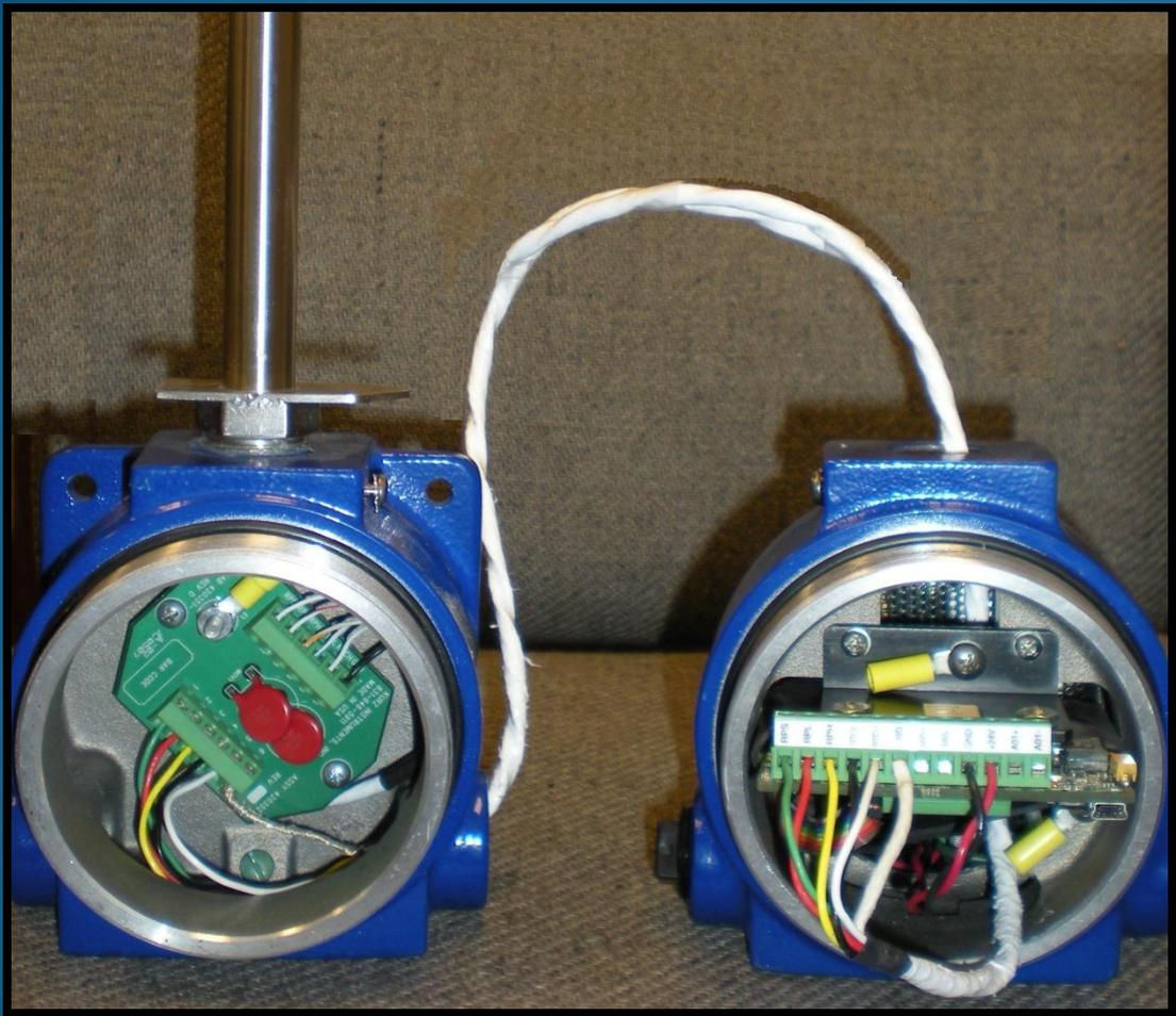
Example with short run of sensor cable attaching the electronics enclosure to the sensor junction enclosure
