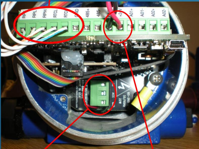
Terminal strip for customer's AC power input
