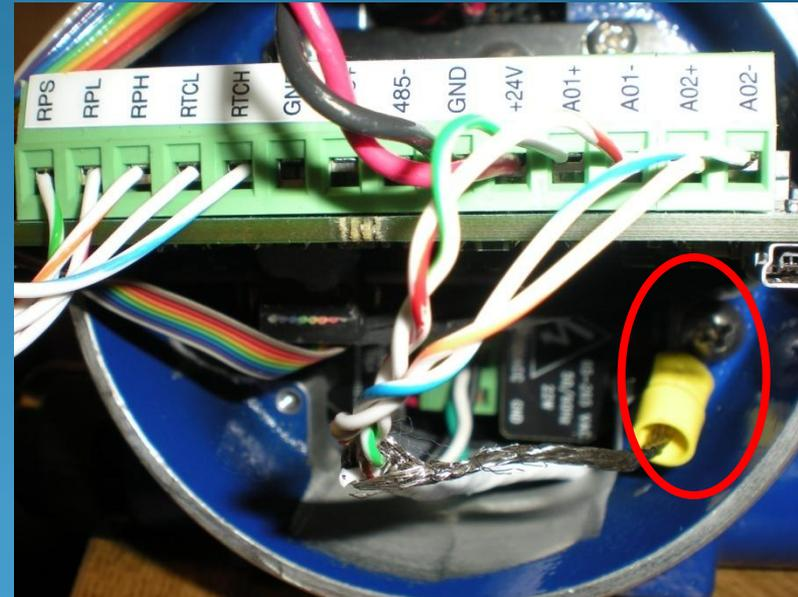
Typical 4-20mA field wiring termination
