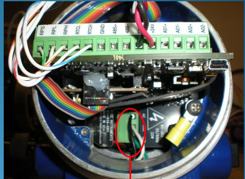
AC power field wiring installed
