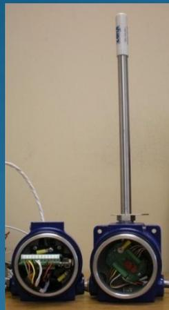
The paired enclosures must have matching sensor serial numbers as shown on the product label
