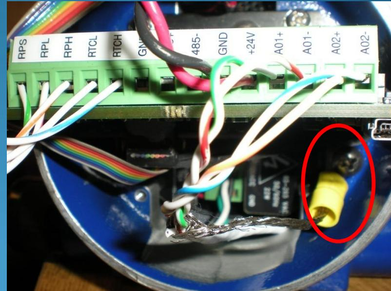
Typical 4-20mA field wiring termination
