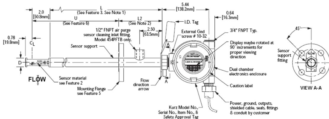
Figure AE-1. 454PFT Flow Meter. Note the 1/2" compressed gas port between the flange and electronics head for purge cleaning gas.
