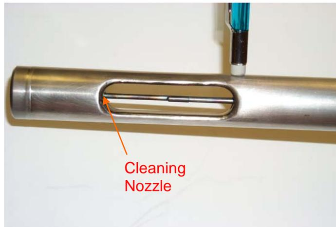
Figure AE-2. Typical purge sensor and window.
