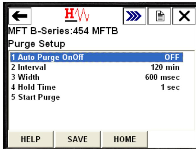
If the Purge Timer has been turned ON, the purge cycle initiated through the HART interface will not affect the purge sequence controlled by the internal timer.
