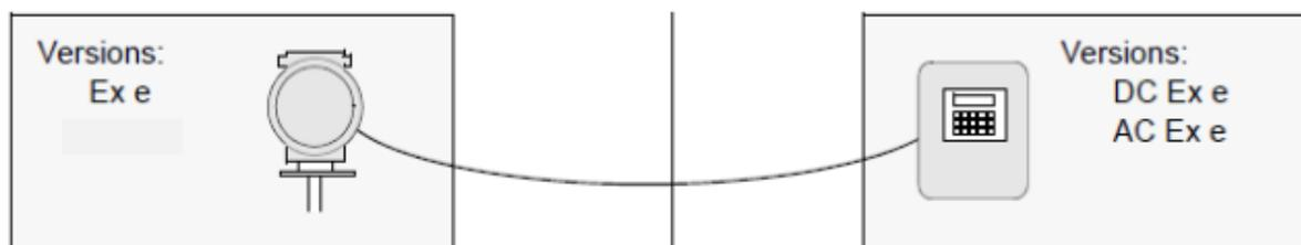
**Image 3.** Transmitter Separate Configuration with polycarbonate enclosure
