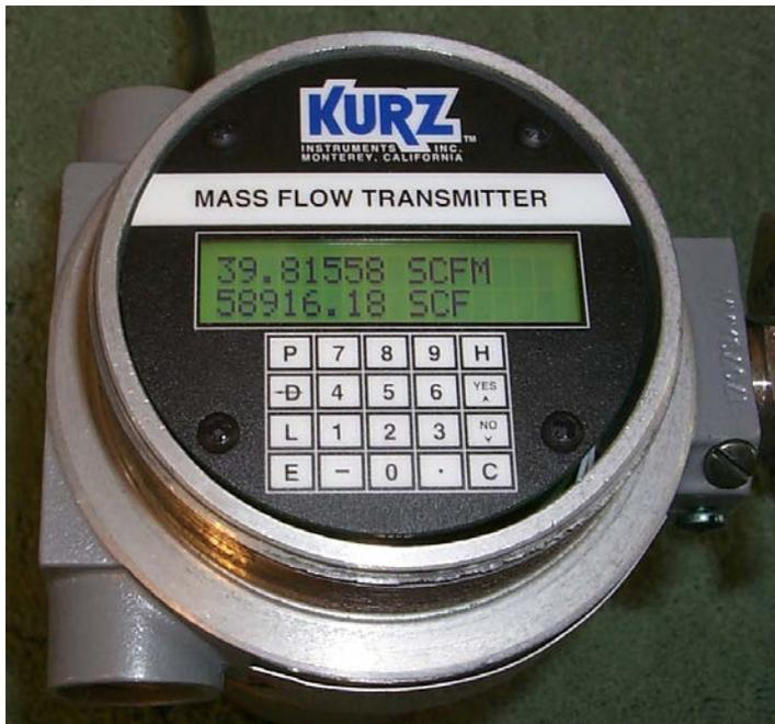
Figure 2. Optional Keypad/LCD. A small finger or pencil eraser works best to hit the membrane keypad in the center of each key. This display will mount on any 90 ° angle within the enclosure. Shown here with the flow body to the right and power/signal conduit ports on the top and bottom.
