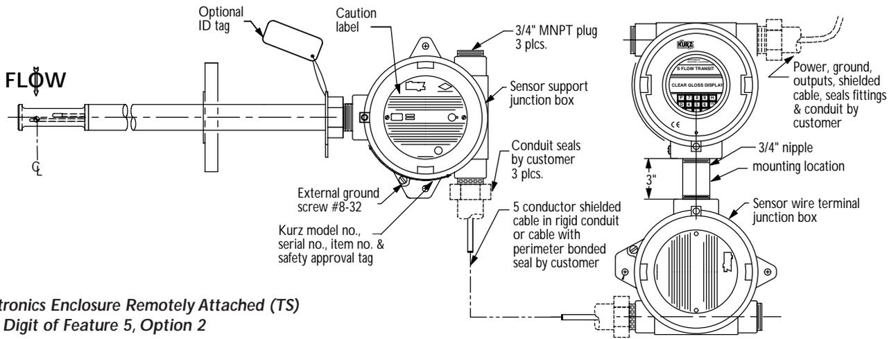
**Electronics Enclosure Remotely Attached (TS)**
