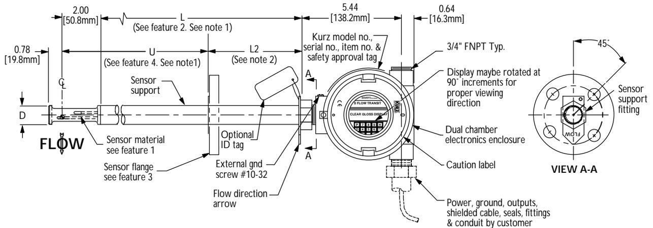
**Directly Attached Electronics Enclosure (TA)**
